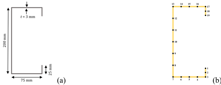
Figure 6. (a) Geometry of a lipped channel section and (b) utilised FS discretisation
