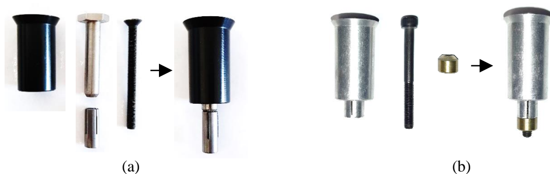
Figure 2: Dismantled and assembled connectors: (a) Type 3 and (b) Type 4 [14]
